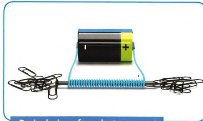
Basic design of an electromagnet
