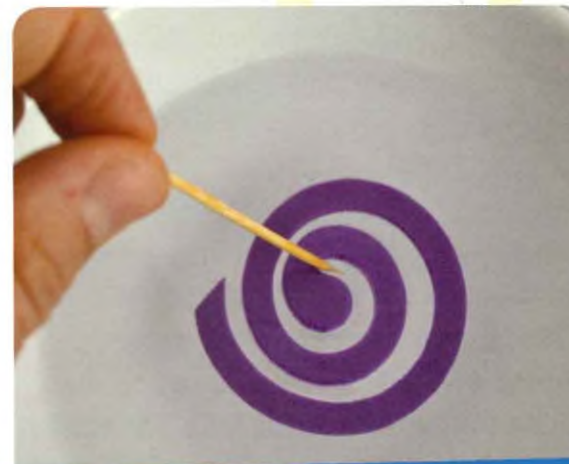
The spiral starts to rotate as soon as you stick the dishwashing liquid-coated tip of the toothpick in its center.
