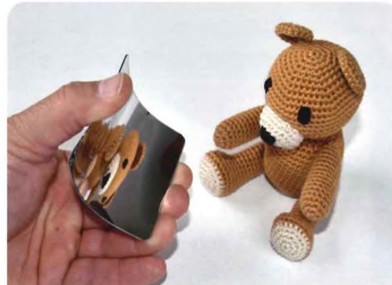
When you bend the mirror inward, the mirror image is suddenly upside down.
