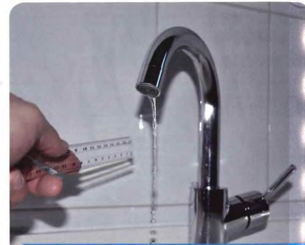
As long as the charged ruler is sufficiently far away, the water runs down in a straight line.
